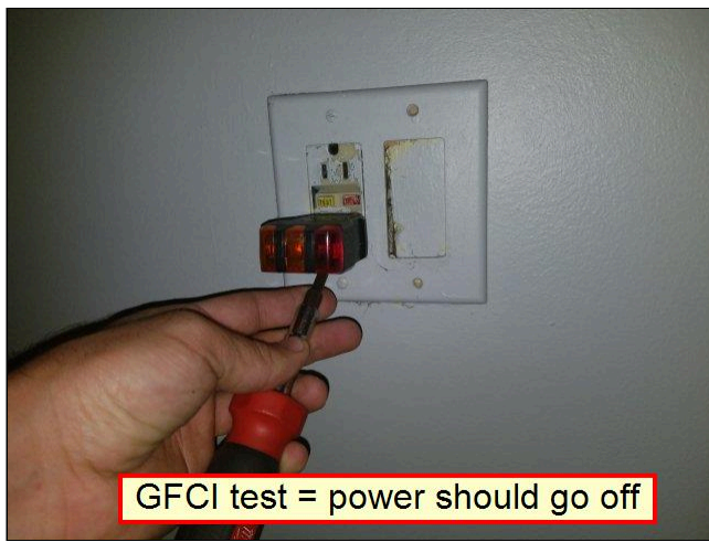
8.6 GFCI TEST Photo 1
