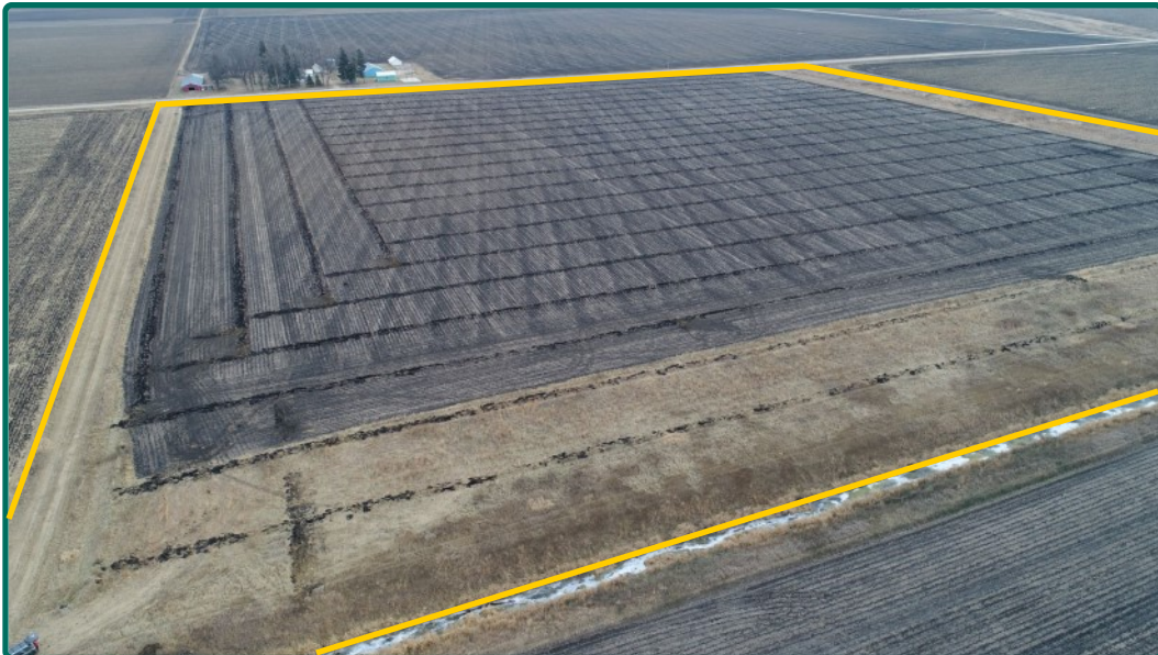
View from northwest corner on December 16, 2017 showing tile trenches
