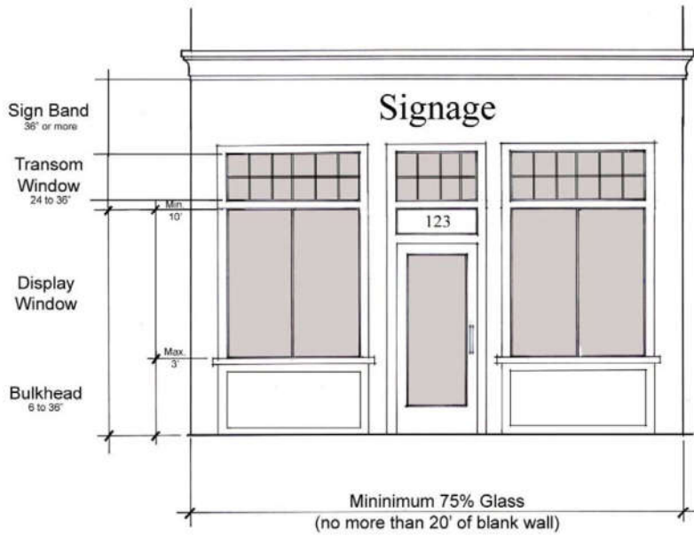
Infill Commercial Storefront on small lot
